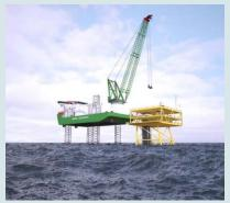
'Gulliver' seagoing sheerlegs 4,000 ton lifting capacity
